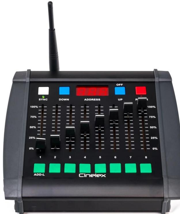
Thank you purchasing the Cinelex Desk-TX8. The DESK-TX8 is an 8 fader portable wireless transmitter using the LumenRadio CRMX standard protocol. It will transmit DMX512 industry standard DMX signals to any LumenRadio compatible wireless receiver such as the Cinelex Skynode or TRX, as well as any other compatible receiver or light fixture.
